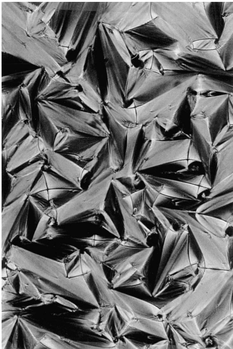
FIGURE 4 Polarizing micrograph of 10 at 337 K, cooled from the isotropic liquid at 2°C/min.
